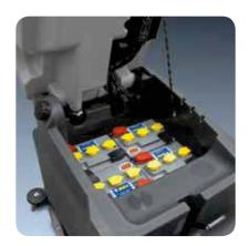
Great working autonomy thanks to the possibility to use 4 batteries 6 V 240 Ah granting continuous working up. Possibility to use also 2 batteries 12V. Less battery consumption thanks to rear wheeldrive. Large load tanks made of shock and acid proof polyethylene (real load of 85 l.), avoiding frequent stop for refilling.
